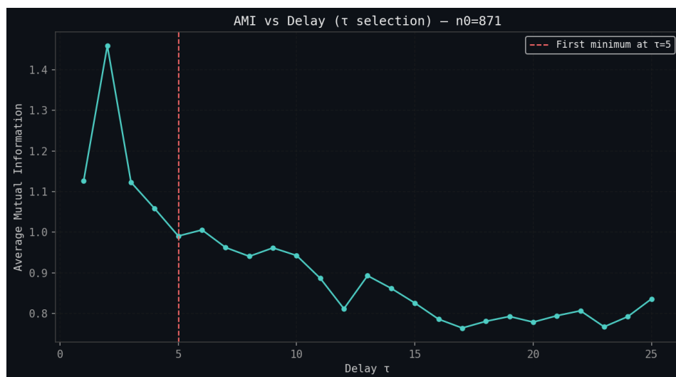
Figure 3: Average mutual information as a function of delay \tau for the longest trajectory ( n_0 = 871 ). The first local minimum at \tau = 5 (red dashed line) is the recommended delay. At this lag, consecutive delay coordinates are maximally independent, satisfying a necessary condition for a good embedding.
